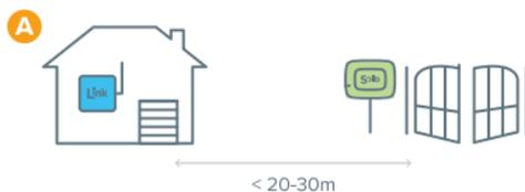
A) 1Control SOLO placed near the gate and 1Control LINK placed in the house on the window closest to the gate. This solution allows you to open the gate both using Bluetooth and using Wi-Fi.
