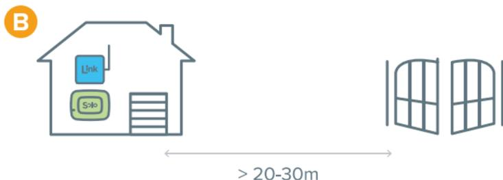
1Control SOLO and 1Control LINK both placed in the house on the window closest to the gate. In this way, taking advantage of the operating range of the remote control copied into your SOLO, it is possible to cover a greater distance and open through the Wi-Fi.
