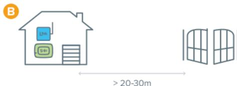
B) 1Control SOLO and 1Control LINK both placed in the house on the window closest to the gate. In this way, taking advantage of the operating range of the remote control copied into your SOLO, it is possible to cover a greater distance and open through the Wi-Fi.
