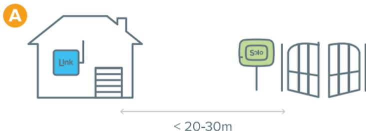
1Control SOLO placed near the gate and 1Control LINK placed in the house on the window closest to the gate. This solution allows you to open the gate both using Bluetooth and using Wi-Fi.
